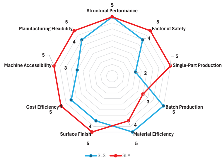
Fig. 2 Comparative performance of SLS and SLA based on the proposed Manufacturing Decision Framework.
