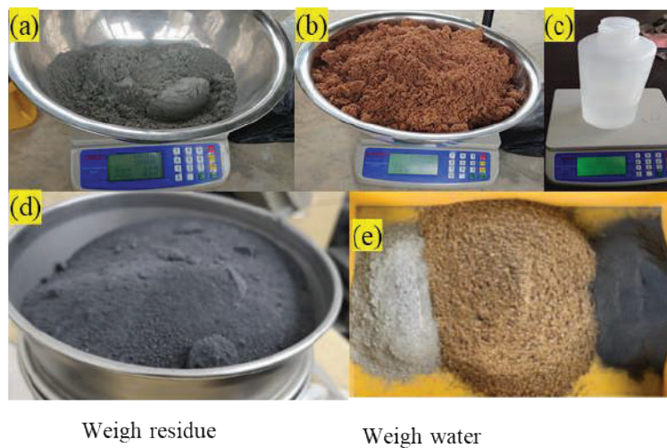
Fig. 1 Material for mixing cement sand brick: (a) Weigh cement, (b) Weigh sand, (c) Weigh water, (d) Weigh treated SW501 residue and (e) Mix all material
