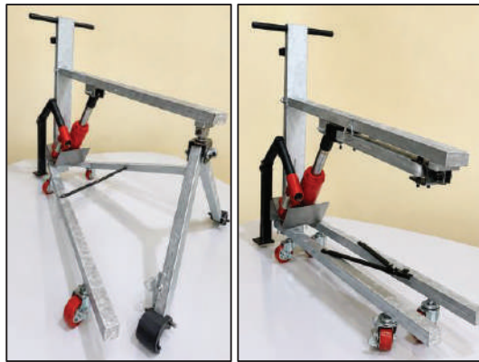
Fig. 2 Final Prototype of the Proposed Manhole Cover Lifter (Expanded on the Left and Folded on the Right).
