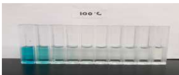
Figure 3 MB solution color changes by presence of KF-TiO 2 (0,15,30,45,60,90,120,150,180 and 1140 minutes)
