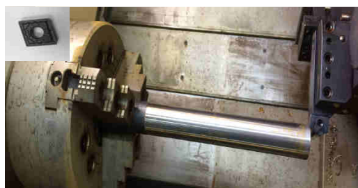
Figure 1 SANDVICK Coromant cutting tool setup inside CNC Machine DMG- CTX 310
