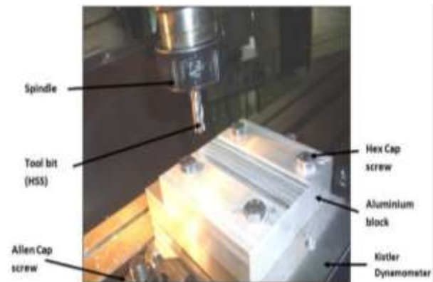
Figure 2 Aluminium block during milling operation
