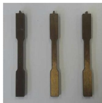
Figure 1 Tensile test sample
