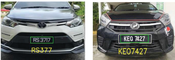
Figure 4 Misleading characters of number plate
