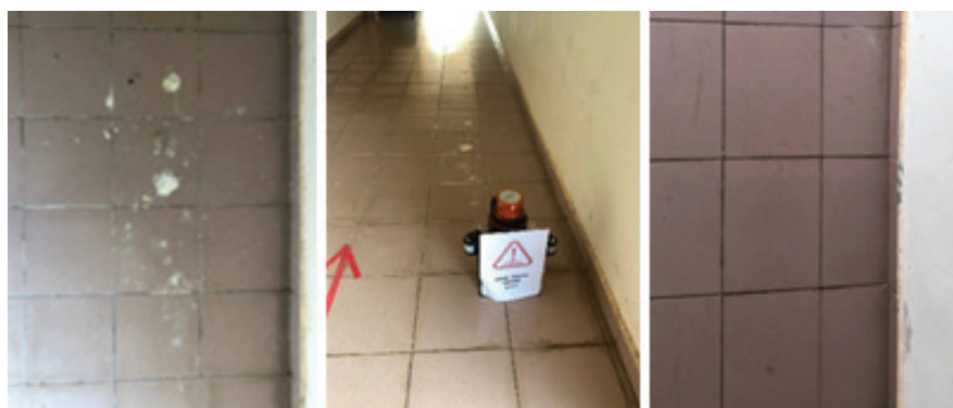
Figure 8: Before and After Installing Infrared Bird Repellent Sensor on the Sidewalk B
