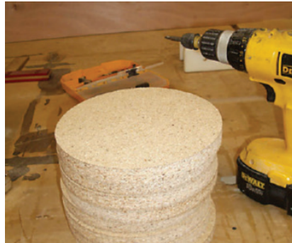
Figure 3: Kenaf core particleboard for sound absorption test [16]
