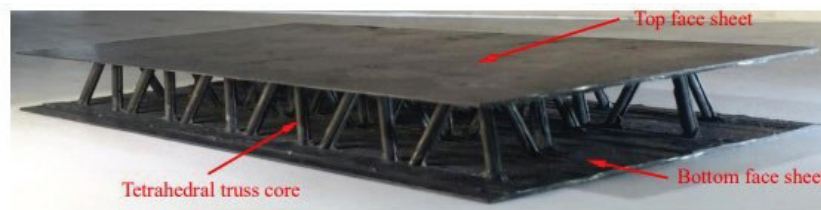
Figure 1: Composite sandwich panel with tetrahedral truss structure core [6].
