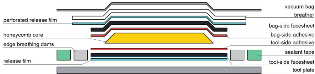
Figure 4: Schematic of sandwich panel layup [13]
