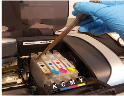
Figure 3: Nano-silver ink and aqueous vehicle filling process into the CMYK empty cartridges of an Epson Stylus C88+ inkjet printer
