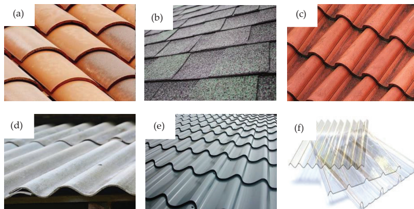
Figure 3: Type of roofing material (a) clay [7], (b) asphalt [8], (c) concrete [10], (d) asbestos cement [12], (e) metal [14], (f) polycarbonate [15]
